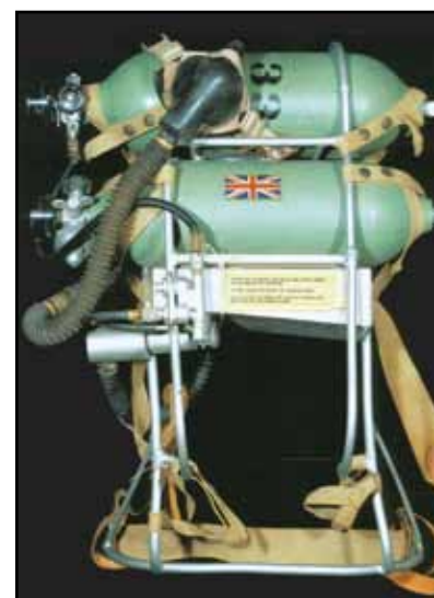
Figure 3.6: The oxygen apparatus used on the first successful ascent of Everest in 1954, with the oronasal mask which can be seen strapped to the upper cylinder.
