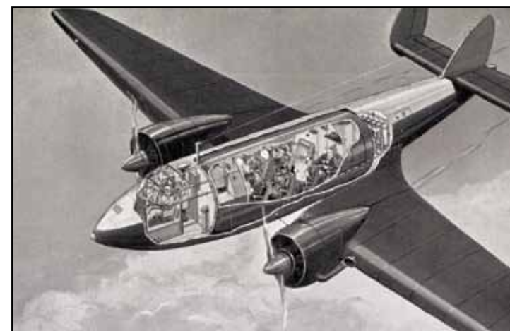
Figure 6.2: Haldane's design for a pressurised aircraft drawn in the 1920s.
